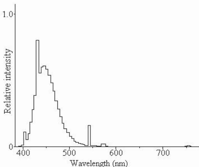
Fig. 2. Spectral characteristics of lamps emitting blue light by Philips (TLD 36W/18)
