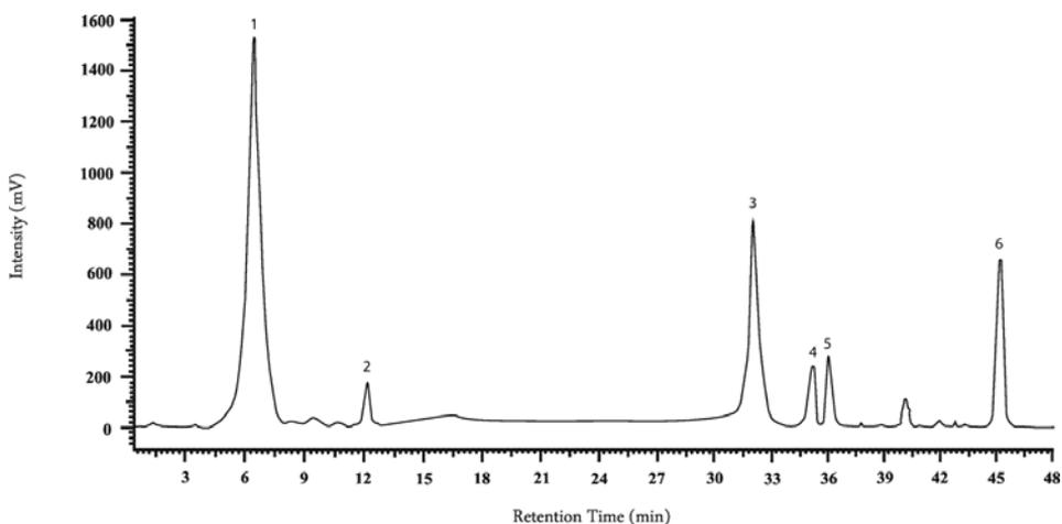
Fig. 2. HPLC chromatogram of extract from fruiting bodies of *Boletus badius*: (1) protocatechuic acid, (2) *p*-hydroxybenzoic acid, (3) *p*-coumaric acid, (4) ferulic acid, (5) sinapic acid, (6) cinnamic acid
