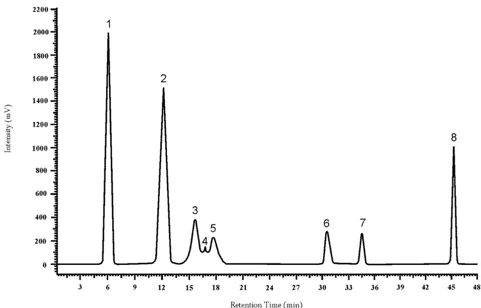
Fig. 1. HPLC chromatogram of standards of selected phenolic acids: (1) protocatechuic acid, (2) *p*-hydroxybenzoic acid, (3) vanillic acid, (4) caffeic acid, (5) syringic acid, (6) *p*-coumaric acid, (7) ferulic acid (8) cinnamic acid
