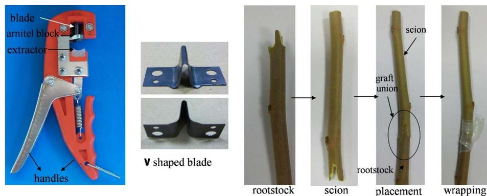
Fig. 1. Manual wedge grafting cut grafting, and grafting processes (Manuel Grafting 3T Art. AR-INN3T, made in Italy, by Arti Tec Company)
